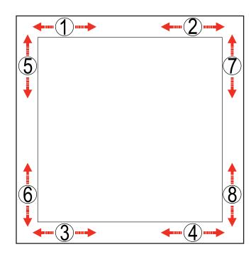
Once the middle of sides are attached, fully press the silicone welt into the channel, between center and corner at location 1. Repeat the process between center and corner at location 2.
