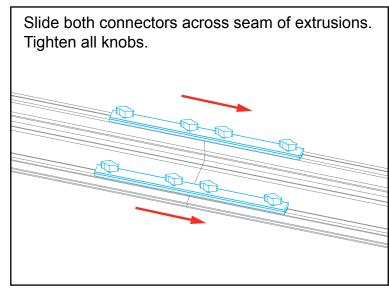
All knobs must be tightened securely to ensure a proper connection.
